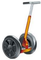
The Segway Human Transporter, also known as the Segway Personal Transporter (commonly referred to as a "Segway"), is a self-balancing, electric-powered transportation device able to turn in place and designed for one person, with a top speed of 20 km/h.
